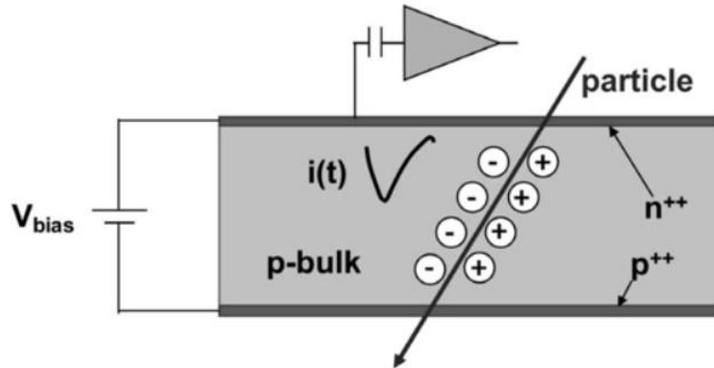
We need electronics to amplify and convert the current signal from the detector into a voltage signal.
