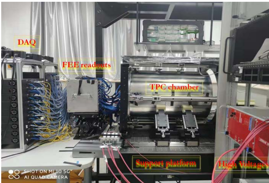
TPC prototype with integrated 266nm UV laser
