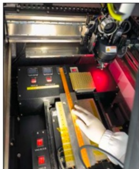
Ladder on wire bonding machine
