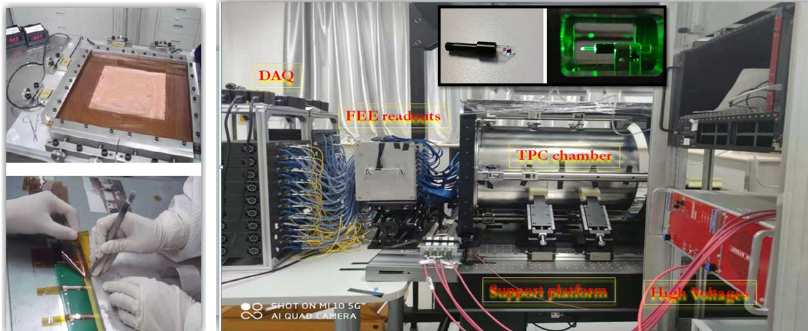
TPC prototype with integrated 266nm UV laser
