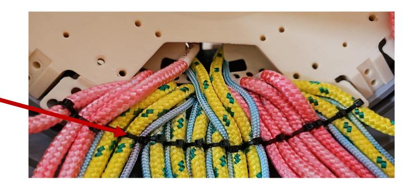
Inner cable holder not serviceable, outer cable holder redesigned to accommodate all cables in pairs
