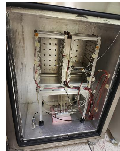
Multi module cold test burn-in setup
