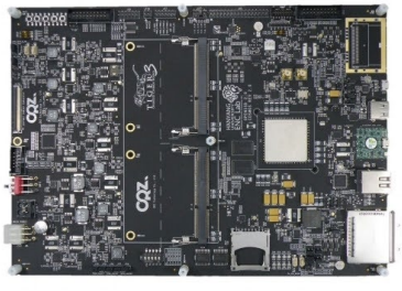
Cosmos/Cosmos+ OpenSSD FPGA Platform
