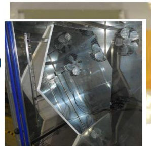
ASTRI-COR3 mirror during Damp Heat test
