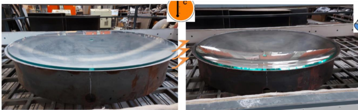
Fig. 2 ASTRI M2 mould + flat glass sheet
