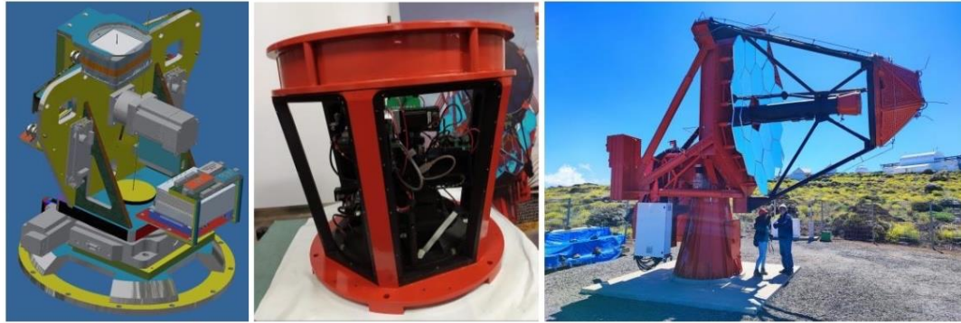
Figure 6. The optical camera. Left: a 3D view showing the main active components of the optical camera. Center: the real object mounted inside the optical camera body. Right: the optical camera mounted on ASTRI-1.
