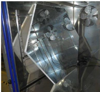
ASTRI-COR3 mirror during Damp Heat test
