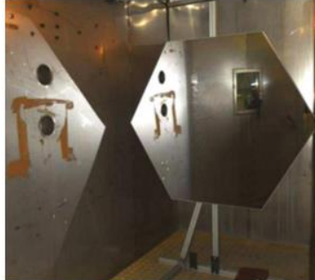
MST mirror in the climatic chamber during the thermal tests
