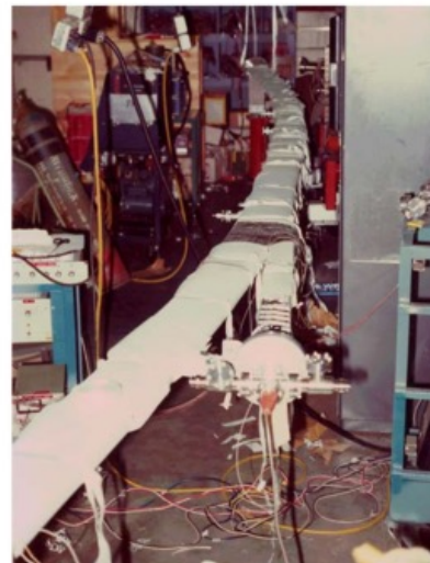
Figure 24. SPEAR bending magnet vacuum chamber with the 1st port to extract synchrotron radiation for experiments (Herman Winick collection)
