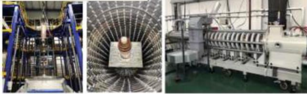
Klystron No. 1 Efficiency 65% (2020)
