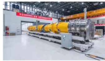
CEPC 1.3 GHz Superconducting Cryomodule (12 m long) (> 100 units needed in China in 5 yrs; CEPC needs 44 units)
