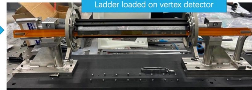
Ladder loaded on vertex detector
