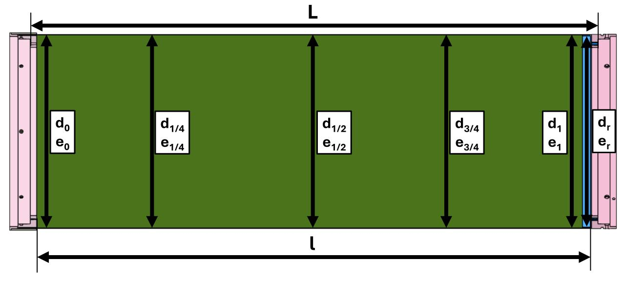
$d_n$  = Diameter at position n  $e_n$  = Ellipticity at position n L = Distance between anchoring points
