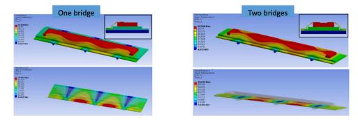
Add a heat sink (HS) to the PCB to enhance thermal conduction, enabling more efficient heat transfer from the ASIC. A heat sink has been applied in JUNO.
