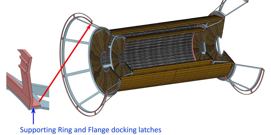
Stave installation for the 3rd ITK Barrel:
