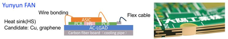
The detailed thermal simulation is ongoing with the heat sink included.
