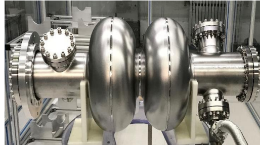
Vertical test of 650 MHz 2-cell cavity
