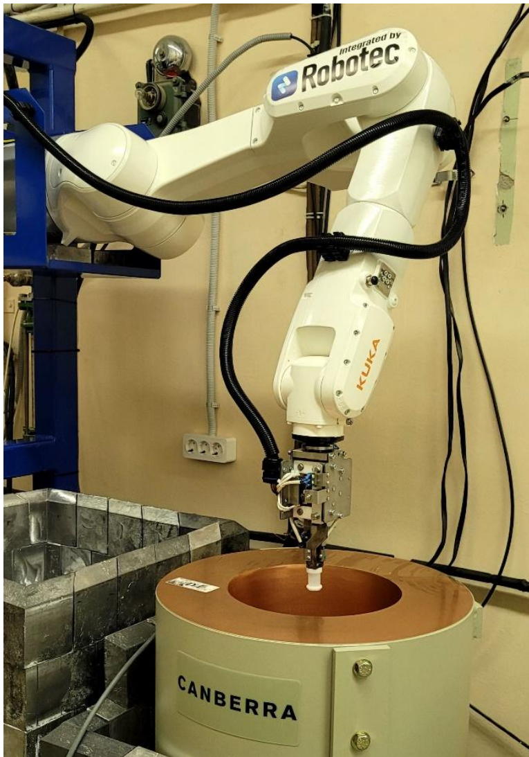
Left photo: KUKA KR 10 R1100 manipulator mounted on a stand. Right photo: Manipulator gripper and cassette holder with containers
