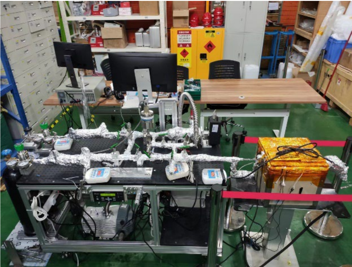
SEOP ^3\text{He} cell filling station (2022)
