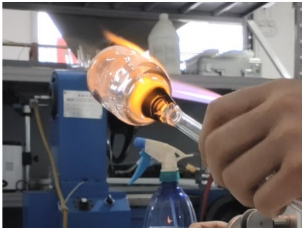
1. In-house ^3\text{He} cell fabrication and filling
