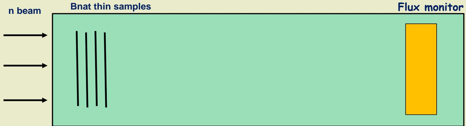
Schematic setup for measuring  $B_{nat}(n,tot)$  xs in the thermal and near-epithermal energy range.
