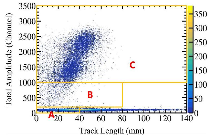
Distinguish fission fragments from  $\alpha$  particles based on both track length and amplitude
