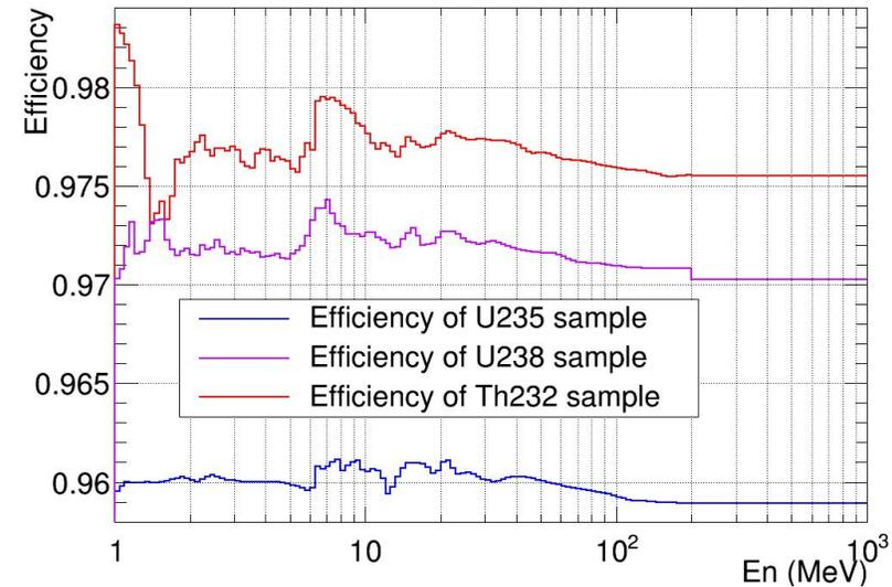
Efficiency determination taking into account the angular distribution of the FFs: the variation due to the anisotropy is less than 1%
