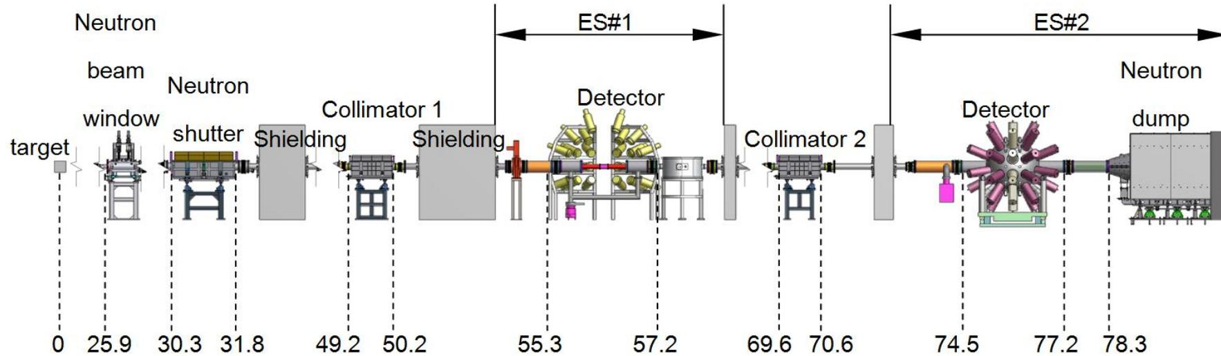
A neutron shutter and two collimators are used together to configure the beam by adjusting their apertures:
