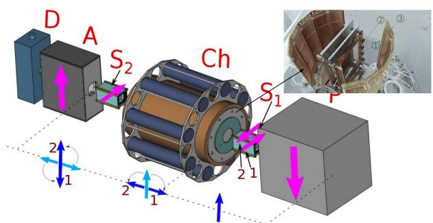
The chamber was filled with CF<sub>4</sub> gas at a pressure of about 10 mbar.
