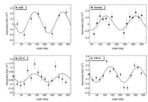
Asymmetry ratio  $D(\theta')$  as a function of the angle for prompt fission  $\gamma$ -rays. The solid line shows the approximation of the obtained angular dependence  $D(\theta')$  by the function  $F = R_{\gamma} \sin(2\theta)$ .
