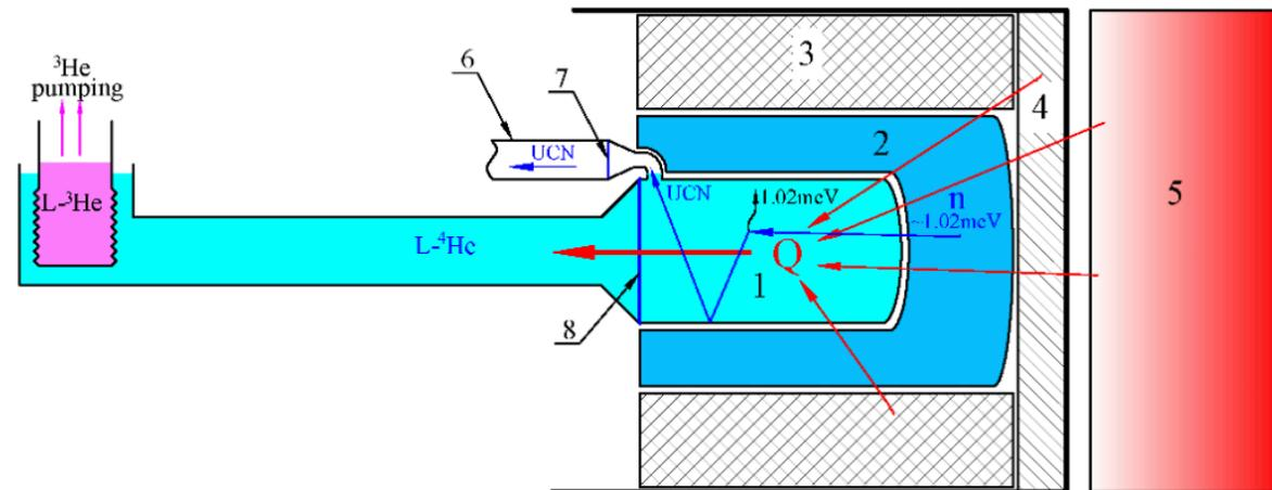
Schematic diagram of the planned ALSUN ultracold neutron source
