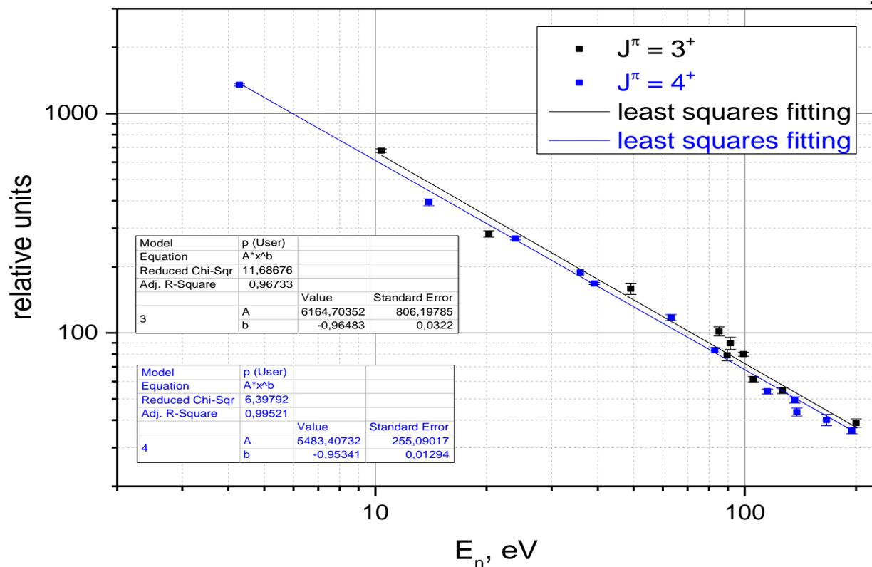
The energy dependence of the neutron flux density obtained from the resonances of the reaction  $^{181}\text{Ta}(n,\gamma)$ . The black squares are for resonances with  $J^\pi = 3^+$ , the blue squares are for resonances with  $J^\pi = 4^+$ ; the lines are LS adjustments. The result is in the 1st row of the table for  $\beta_\alpha$ ,  $\alpha$  is the average value for two spins.
