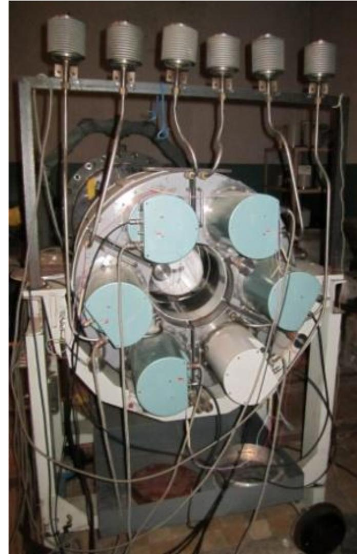
**Large liquid scintillation detector**
