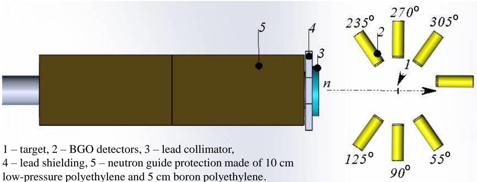
1 – target, 2 – BGO detectors, 3 – lead collimator, 4 – lead shielding, 5 – neutron guide protection made of 10 cm low-pressure polyethylene and 5 cm boron polyethylene.
