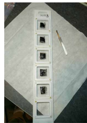
Fig. 4 PGAA sample ladder made of FTPE can accommodate up to six samples measured automatically in one batch in possibly evacuated sample chamber. Five homogenized clay crucible samples (see Fig. 7) are sealed in FTPE foil here. — (© by the authors).
