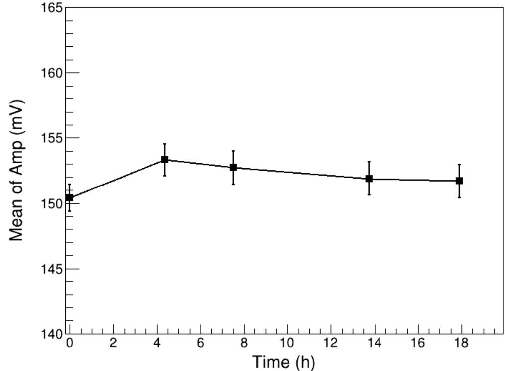
Fig b. Average Amp of LGAD signals under different amount of irradiations
