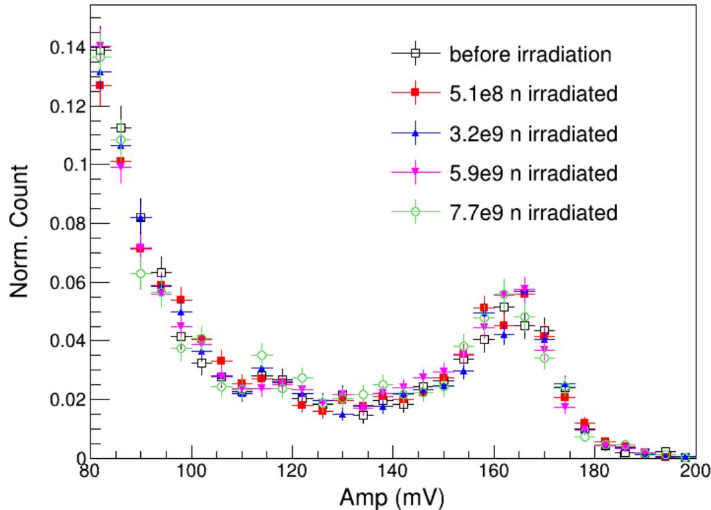
Fig a. Amp of LGAD signal distribution under different amount of irradiations
