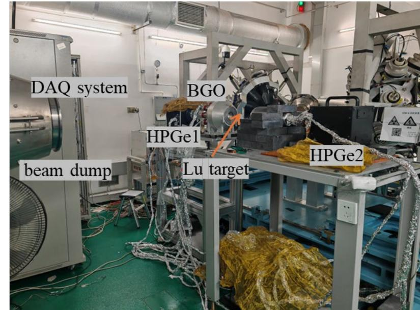
Figure: experimental setup for Lu target.
