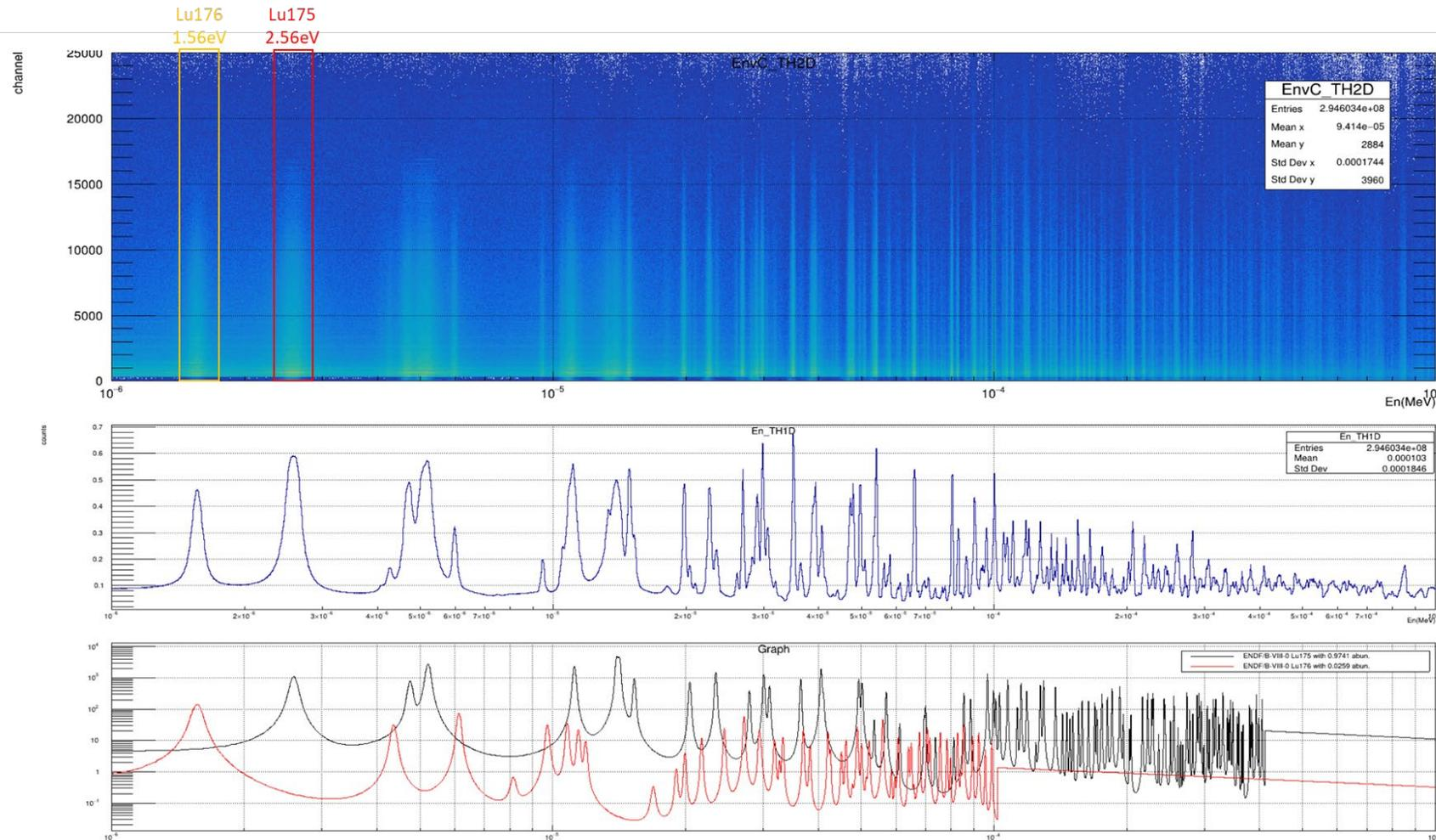
Figure: Lu target results: (top) ToF neutron energy vs gamma-ray energy 2-D spectrum; (middle) ToF neutron energy spectrum; (bottom) Lu ENDF/B-VIII cross section spectrum.
