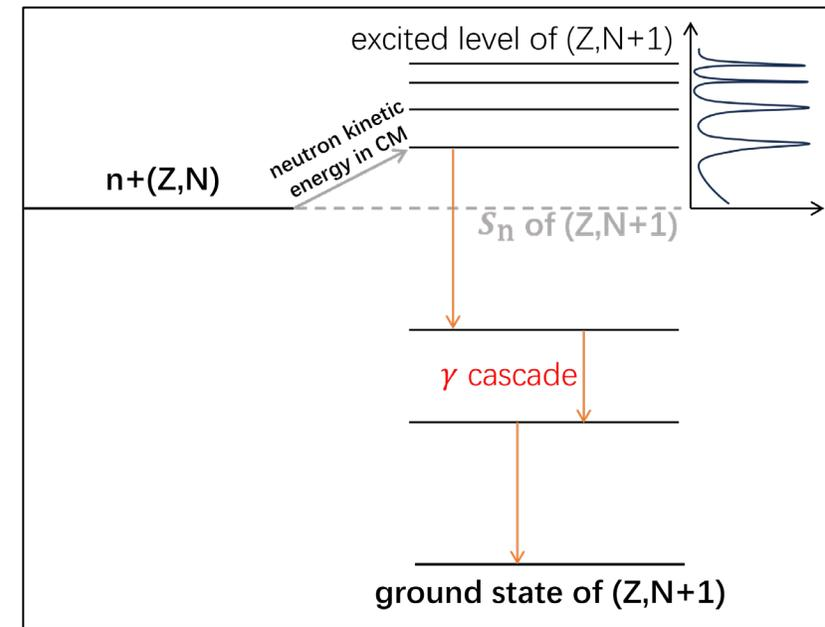
Figure: resonance absorption for neutron
