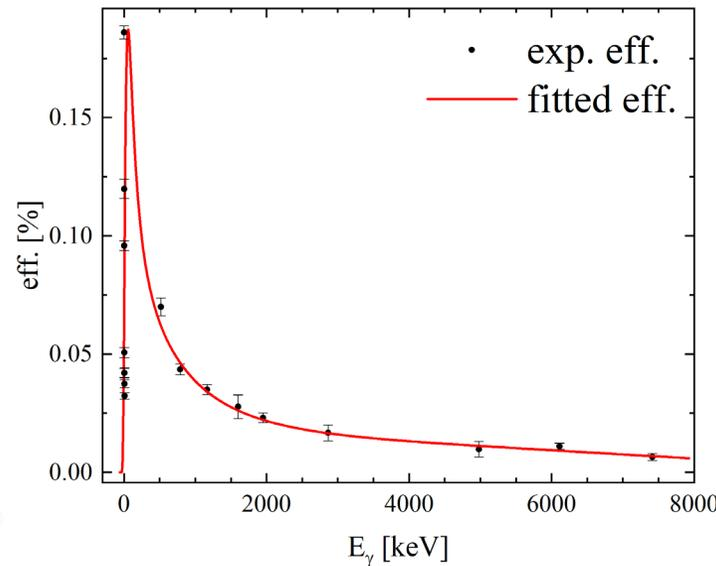
Figure: HPGe efficiency calibration.
