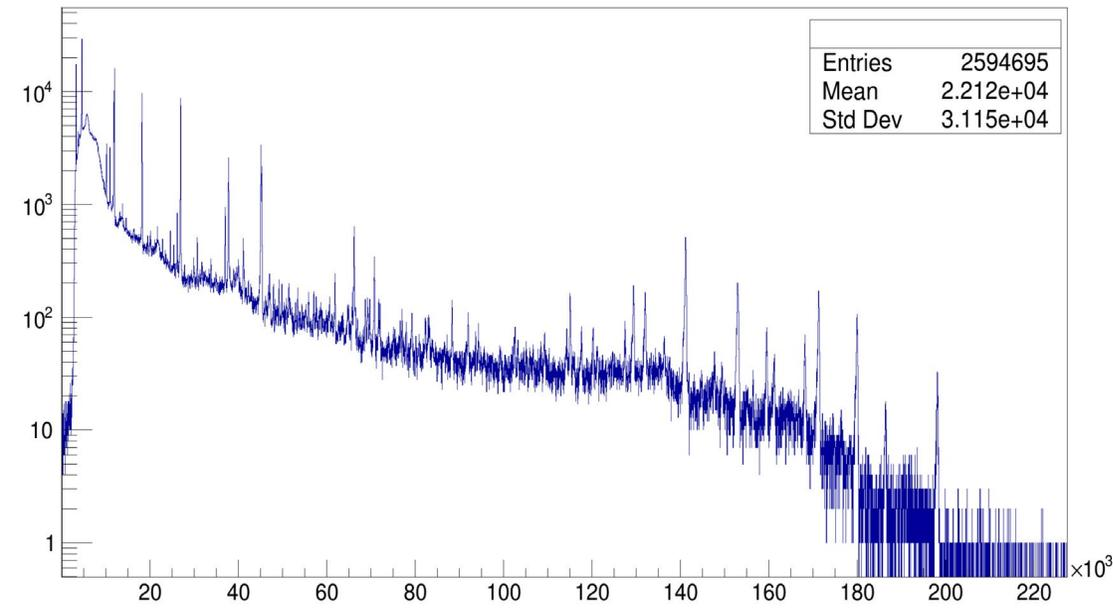
Figure: NaCl gamma-ray spectrum.
