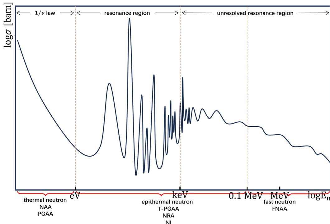
Figure: neutron reaction features for different Noninvasive Techniques.
