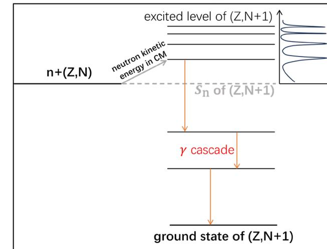
Figure: resonance absorption for neutron
