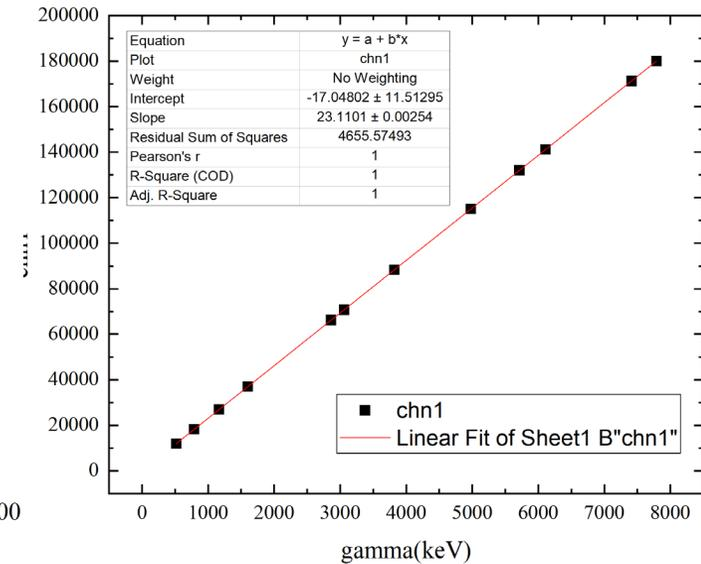
Figure: HPGe energy calibration.
