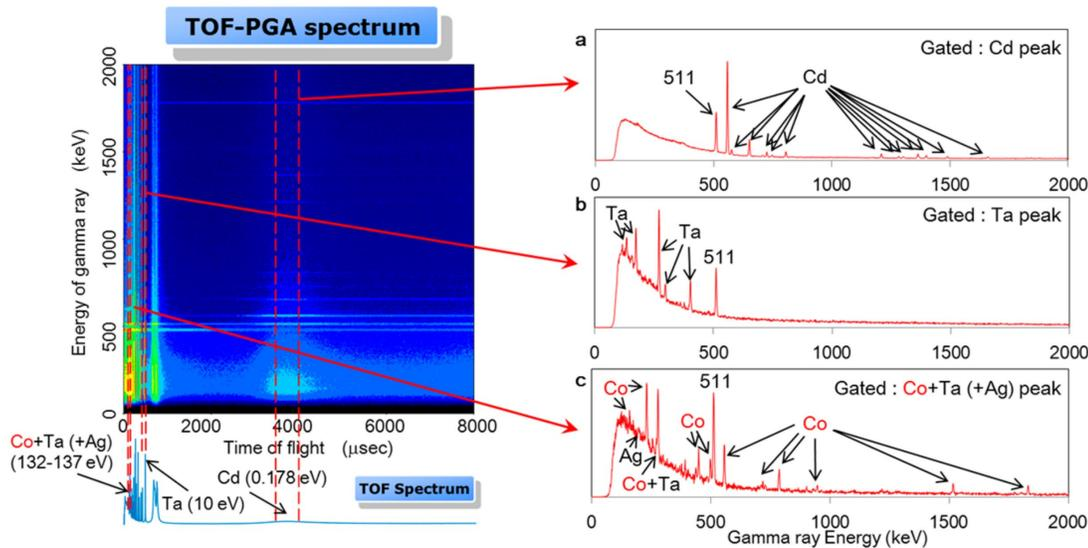
Figure: TOF-PGA spectrum analysis by gating on different gamma-ray peaks.<sup>[1]</sup>
