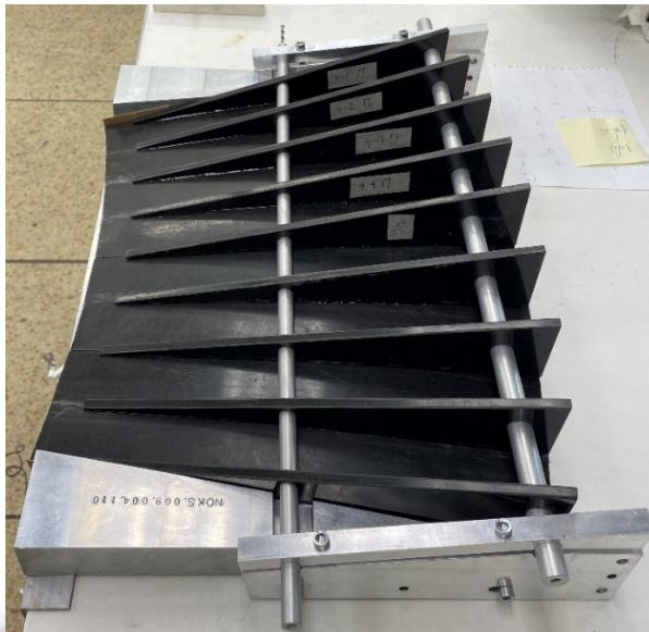
A device for giving the detector body precise geometry, made on a CNC machine
