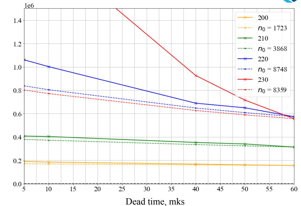
*Neutron count rate with different Discriminator thresholds and dead time*
