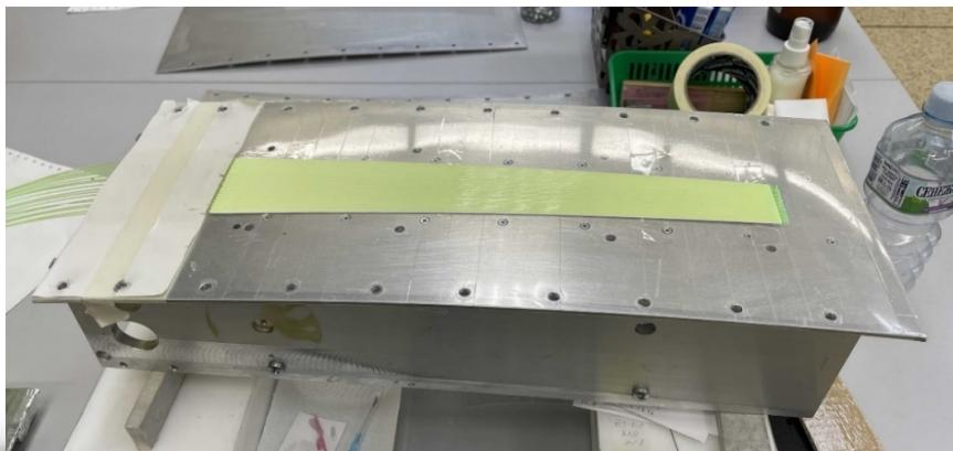
A device for gluing optical fibers in the required bend of the scintillator
