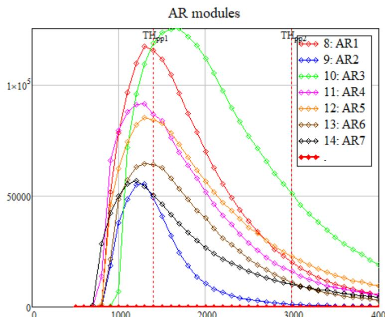
Dependence of high resolution peak amplitude from discriminator threshold value for ASTRA-M counters
