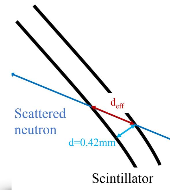
Increased conversion efficiency due to screen placement at an angle to scattered neutrons
