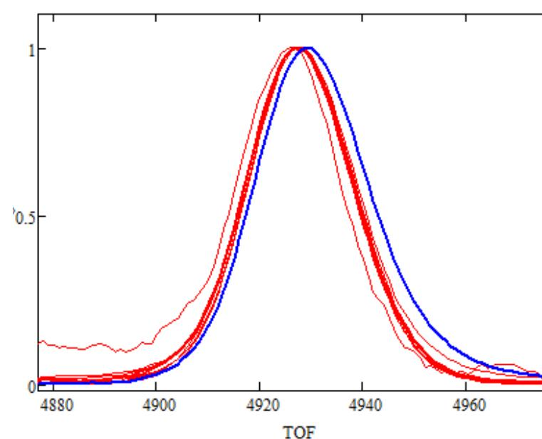
High resolution peak shape for different discrimination parameters
