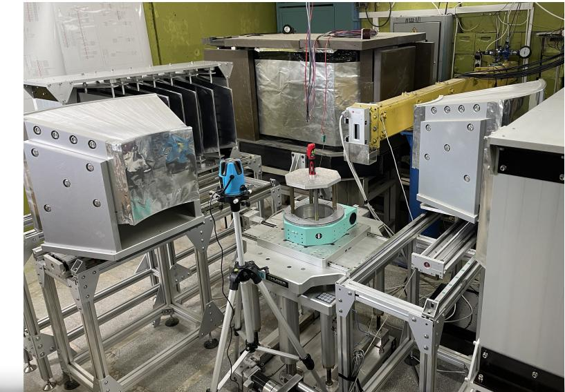
Detector mounted on Fourier-stress diffractometer FSD
