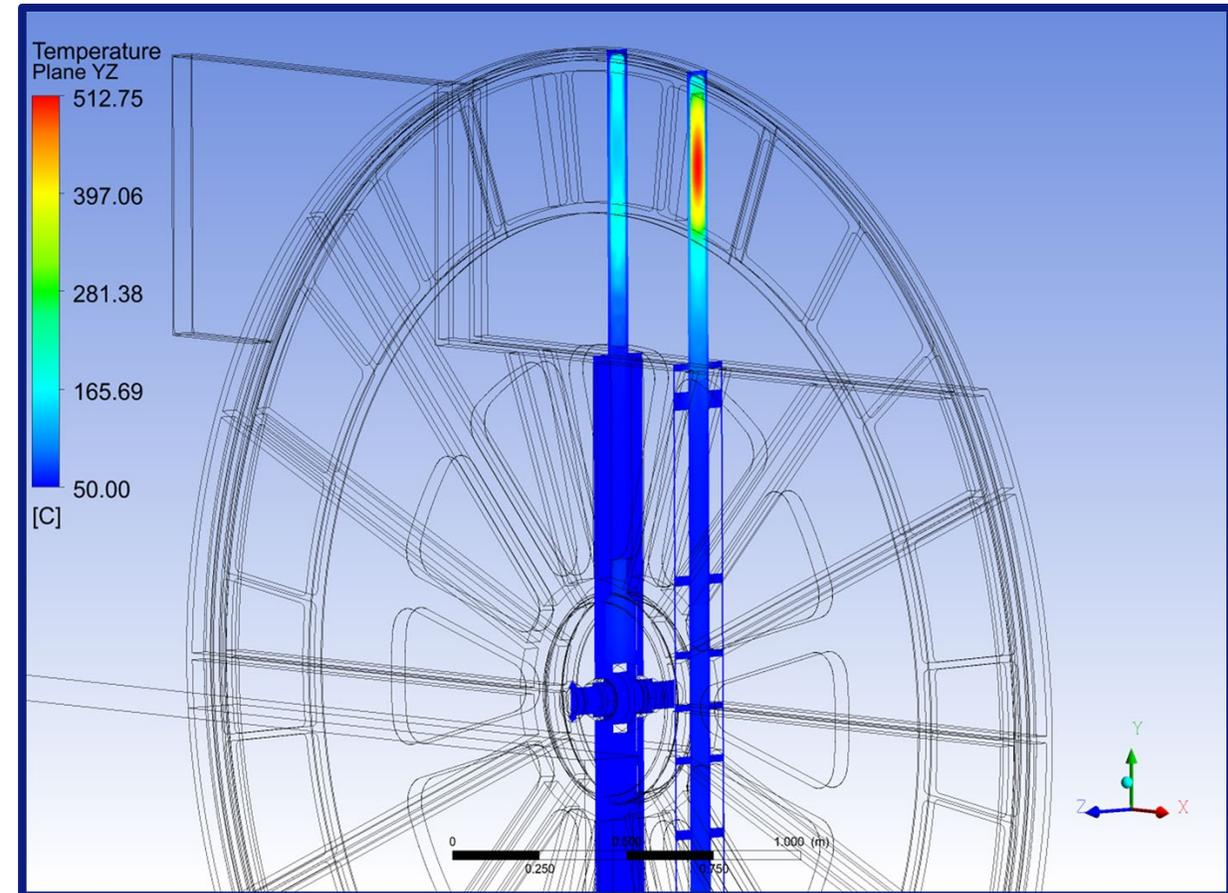
Distribution of the temperature in the RM disc (cross-sections in the YZ plane)
