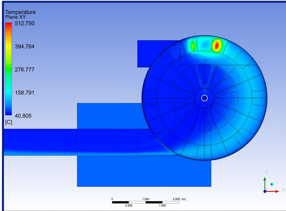
Distribution of the temperature in the RM disc (central cross-section in the XY plane)
