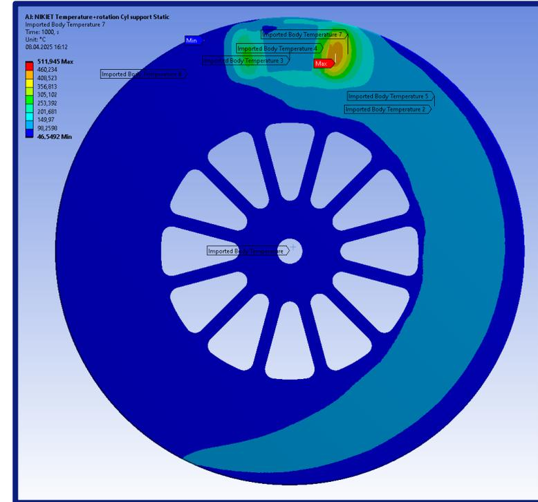
Bearing assembly (1) is modeled using **Cylindrical Support** on the wheel hub surface (tangential movement only).
