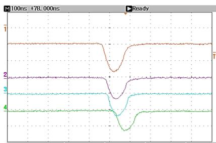
Fig. 2. Beam current oscillograms measured at the control points of the acceleration cycle: 1 - after the 1st section, 2 - after the 2nd section, 3 - after the magnetic spectrometer, 4 - before the target. Oscilloscope sweep -100 ns/div, sensor sensitivity 1 A/V
