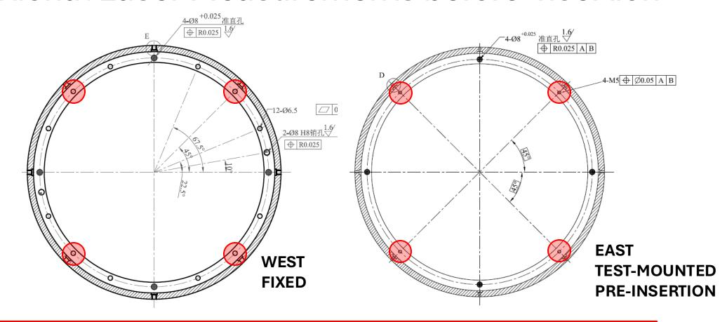
To check alignment of these holes between the two sides
