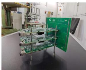
A5202 with 8-layer adaptor board
