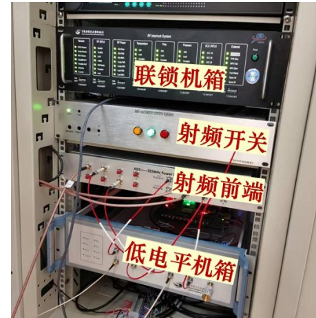
Digital LLRF system Stable operation since 2019
