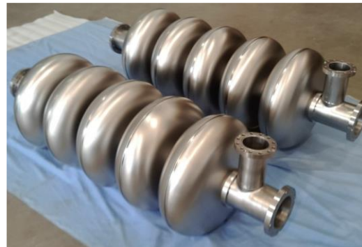
650 MHz 5-cell cavity (beta 0.82)
