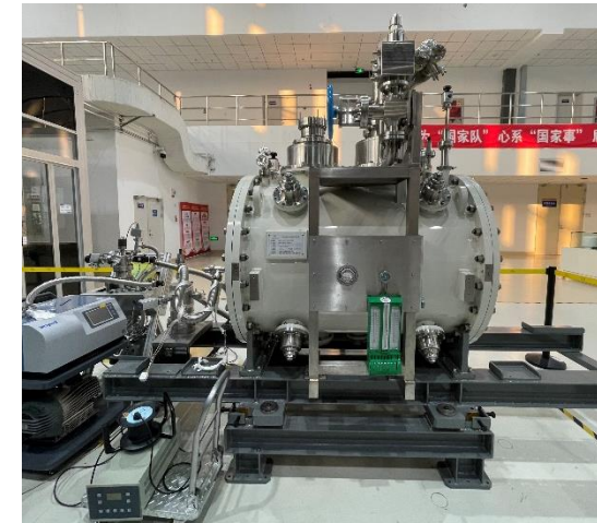
500 MHz KEKB-type single-cell SC cavity module
