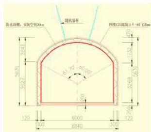
Drill-blast tunnel (6.0m×5.0m)
