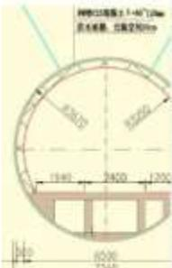
TBM tunnel (D6.5m)
