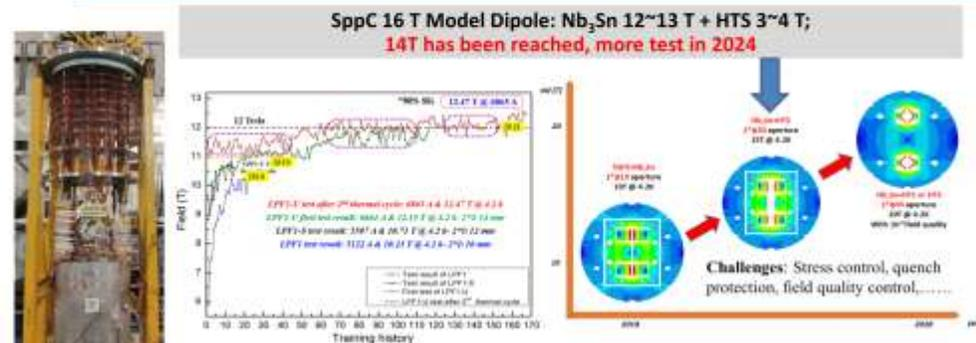
Dual aperture superconducting dipoles achieve 12T@4.2 K and 14T@4.2K entirely fabricated in China. The next step is reaching 16-20T
