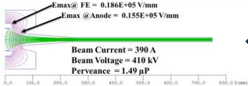
**C band 5720MHz 80MW Klystron design completed**
