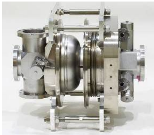
cERL Injector 1.3GHz 2-cell Cavity
