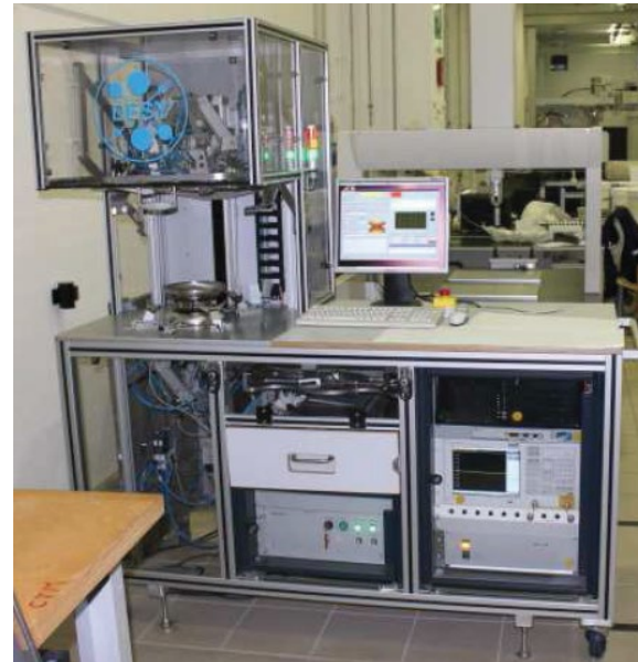
Frequency measurement of half-cell/dumb-bell
