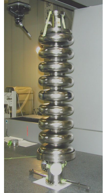
J-ADS 972MHz 9-cell Cavity ( \beta=0.73 )
