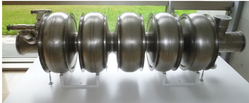
TRISTAN 508MHz 5-cell Cavity
