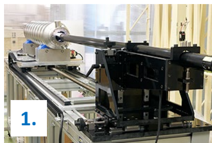
1. Inspection of inner surface
