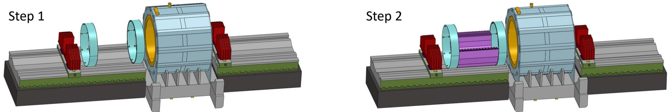
Step 1 : Two auxiliary rings (these two rings are both part of the components, and auxiliary installation tools)
