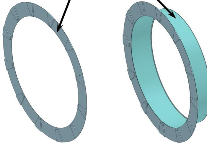
Putting the connection structure of HCAL and Magnet into a computational model
