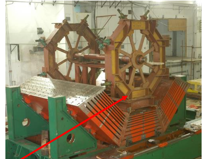
BESIII barrel yoke installation
