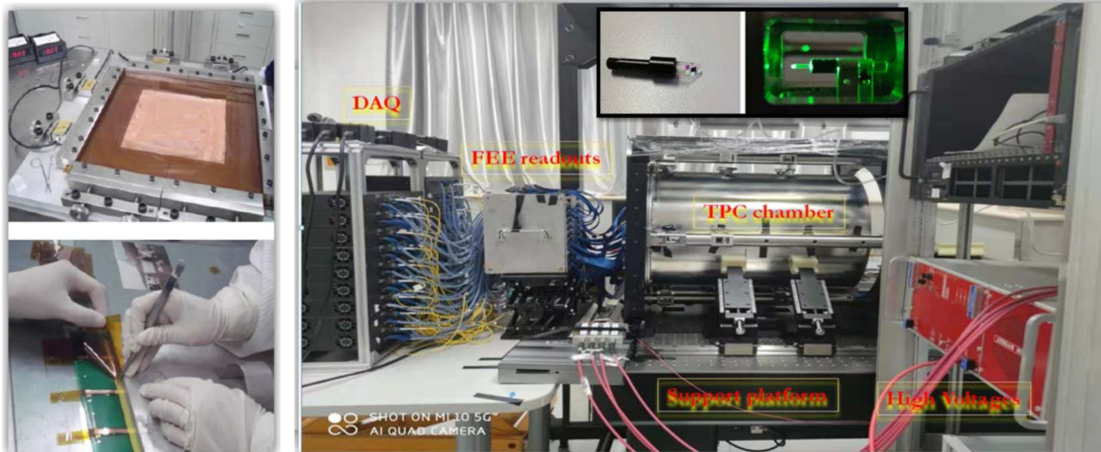
TPC prototype with integrated 266nm UV laser
