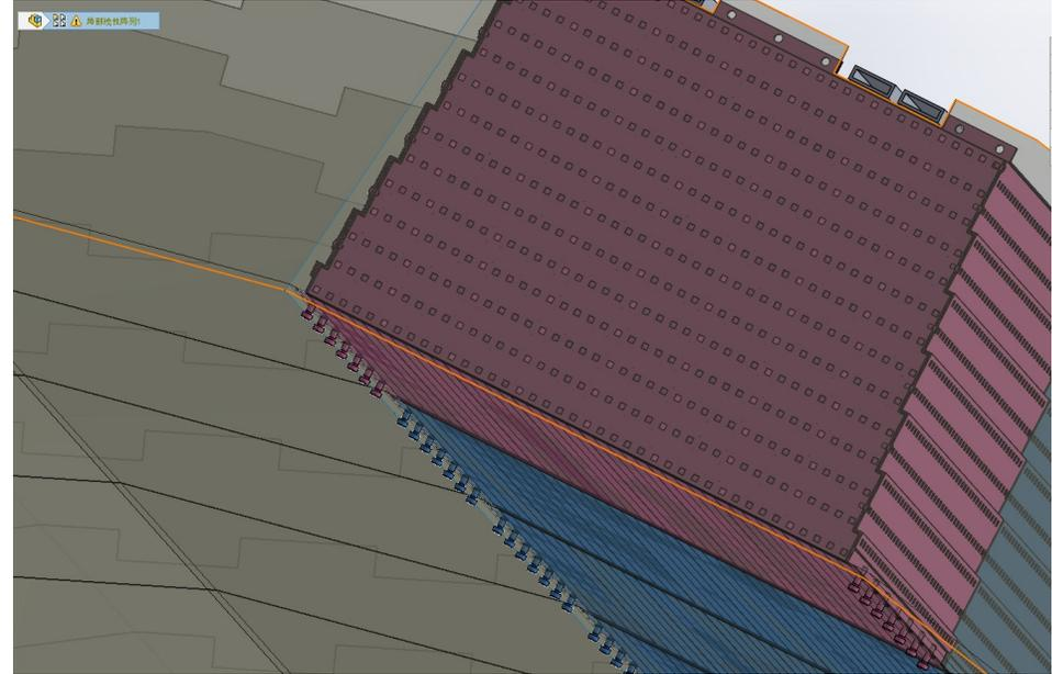
Each module fixed into the main structure by bottom bolts. Four heat dissipation pipes installed at the top of each row of modules.
