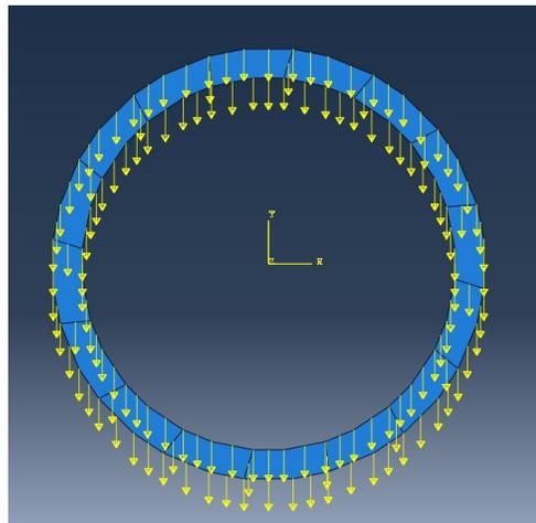
Loads (Gravity+150t static load)
