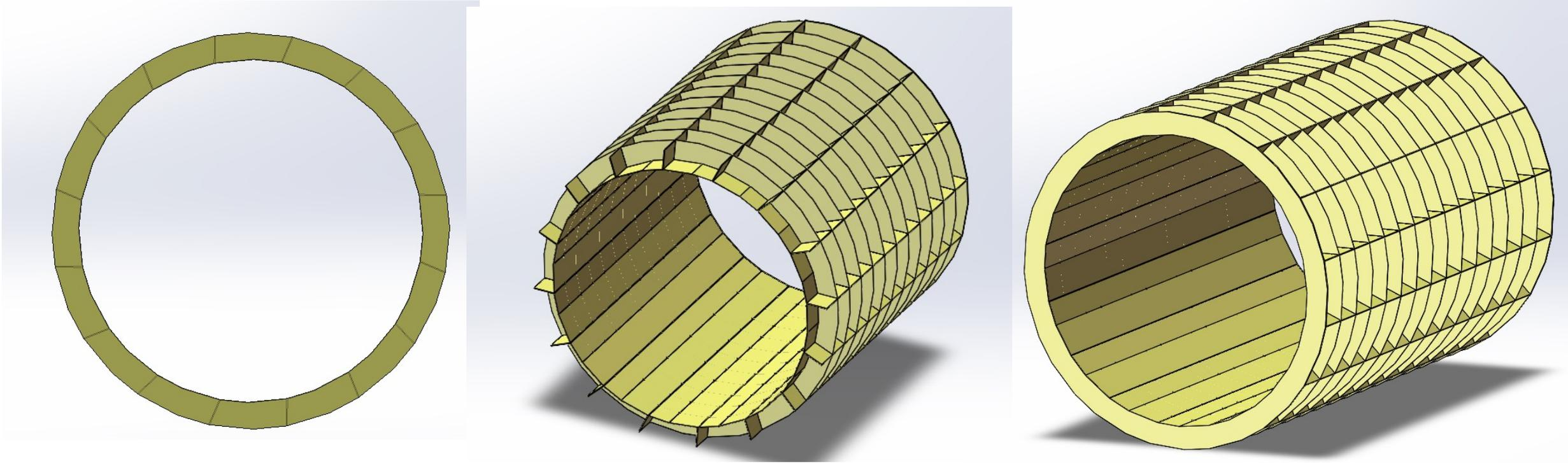
The main structure of ECAL is made of **carbon fiber reinforced epoxy (CFRP)**. The barrel is divided into 16 parts in the ring direction and 15 parts in the Z direction, and each cell has a BGO module.
