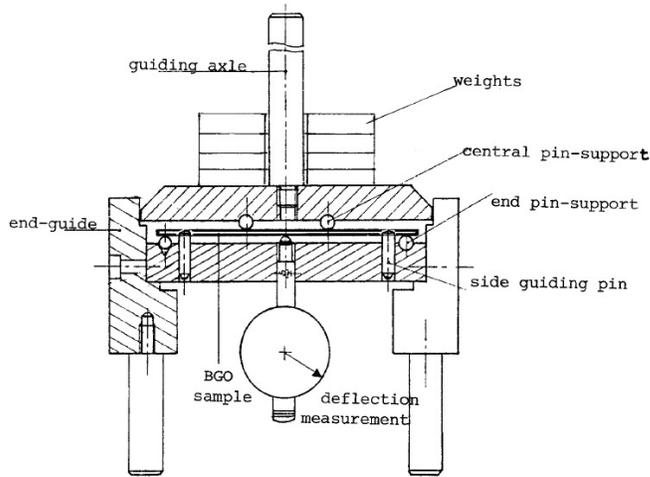
Figure 2 Four-point bending test set-up.
