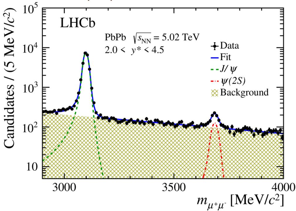
➤ Signal extraction step1: Charmonium yields are extracted from dimuon massfit.
