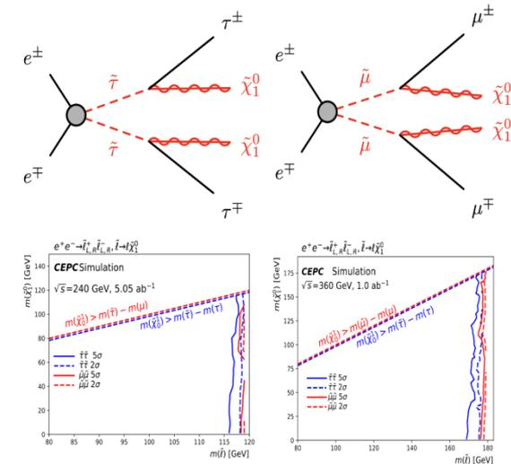
FIG. 60: Top: representative diagram illustrating the pair production of charged staus (smuons) and subsequent decay into a two-tau (two-muon) final state. Bottom: The  $5\sigma$  discovery contour (solid line) and  $2\sigma$  exclusion contour (dashed line) for the direct stau production and direct smuon production with 5% flat systematic uncertainty. Left (Right) plot presents the center-of-mass energy of 240 (360) GeV.
