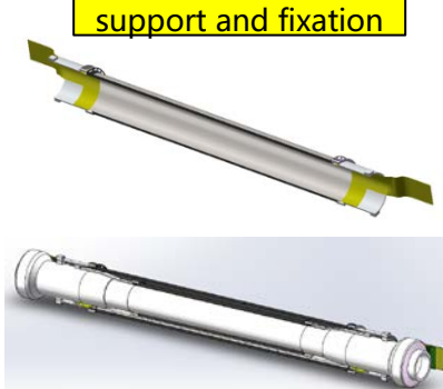
Bent MAPS support and fixation
