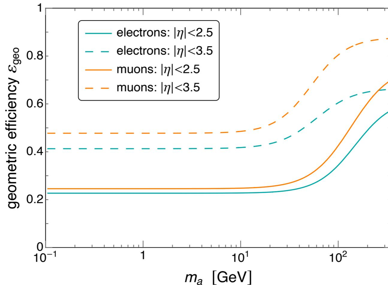
Figure 3: Geometric efficiency of electrons and muons from ALP decays as a function of the ALP mass, for two different designs of the detector:  $|\eta|_{\text{max}} = 2.5$  (solid lines) and  $|\eta|_{\text{max}} = 3.5$  (dashed lines).
