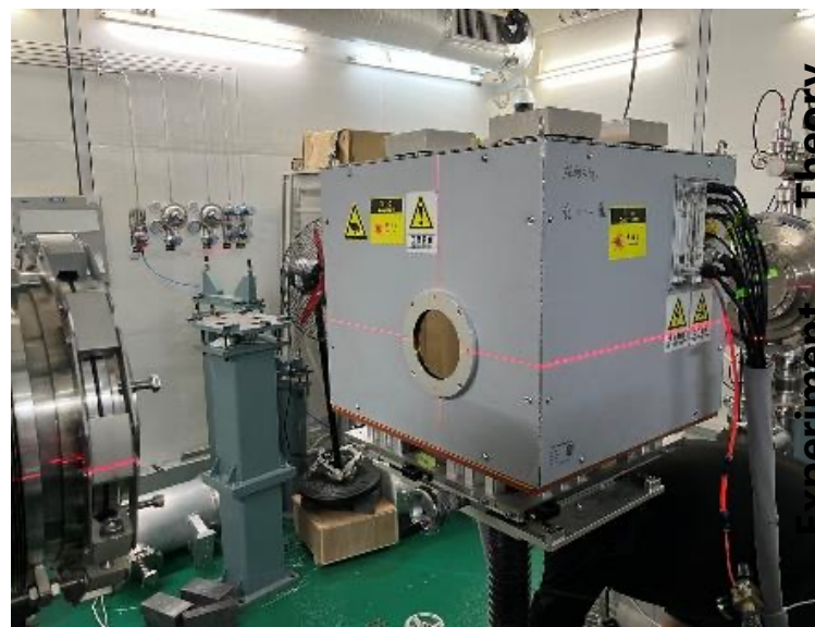
Preliminary setup at CSNS back-n beamline using in-situ ^3\text{He}
