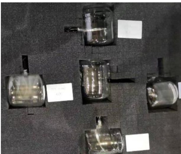
SEOP glass cell containing ^3\text{He} gas
