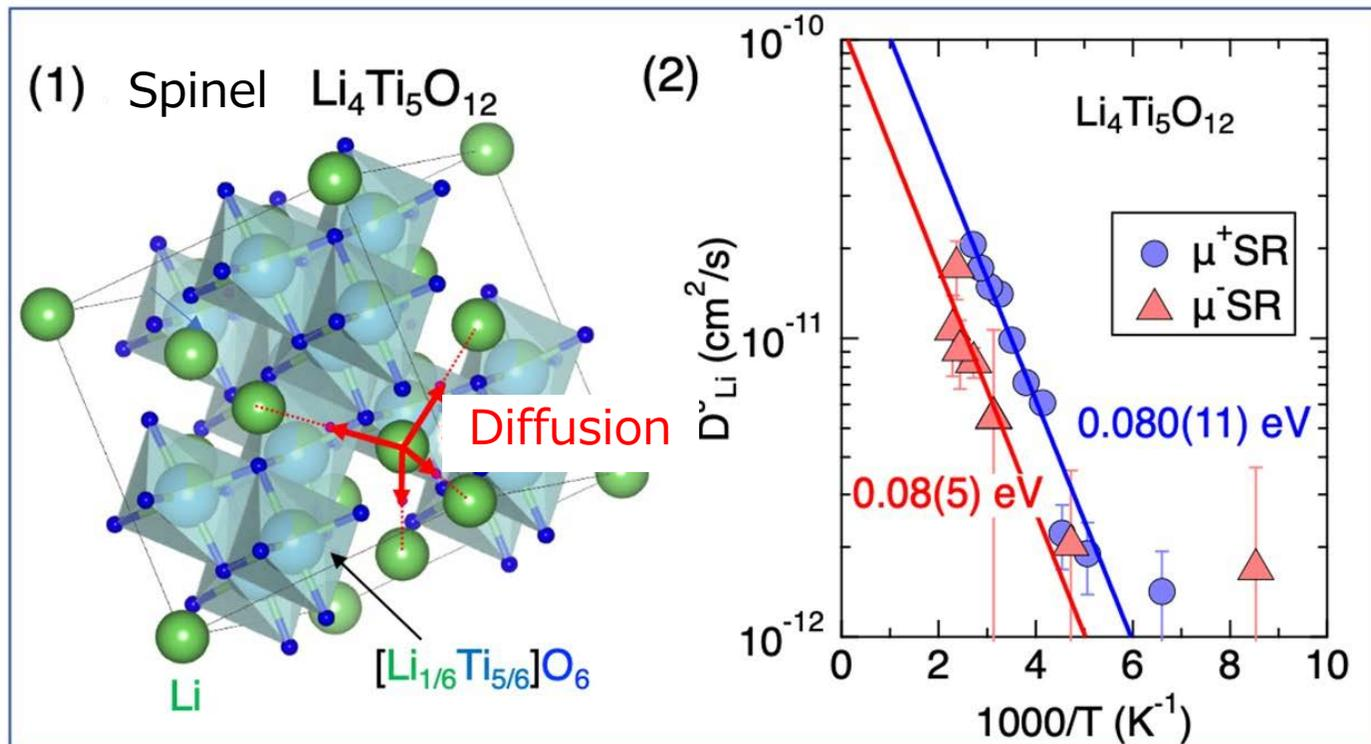
The results obtained with positive and negative muons are both consistent.
