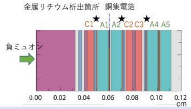
We have already confirmed that we can apply this technique to detect metallic Li. Recently we have started to apply this technique to a cell with multiple pairs of electrode.
