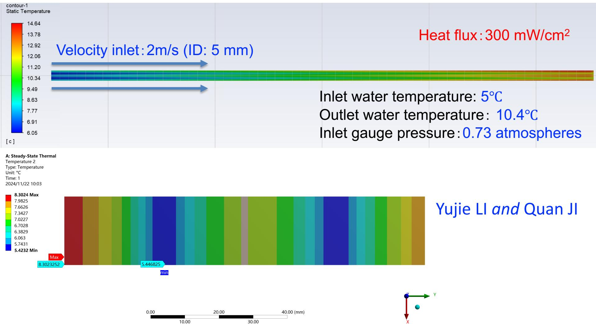
Using a 5 °C, 2 m/s water inlet (ID: 5 mm) from one end, the maximum temperature difference on one sensor is ~2.9 °C.
