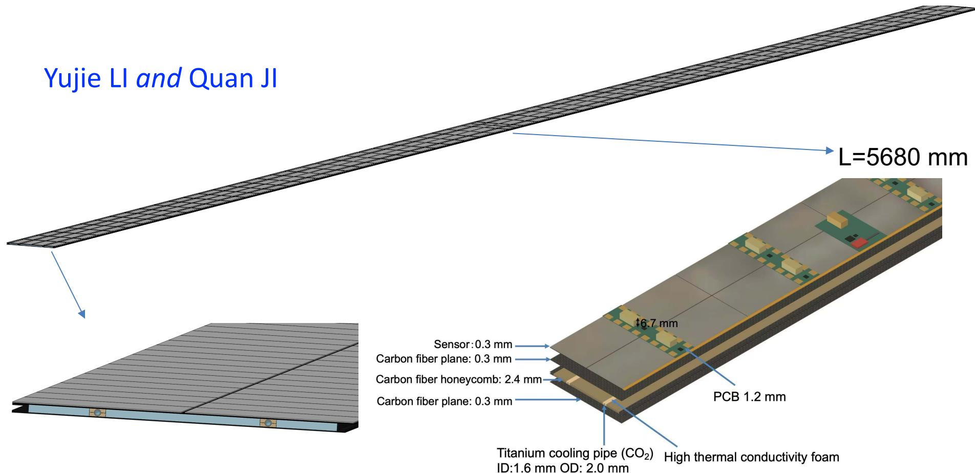
The total height of ladder and its cooling support: 1.12 cm
