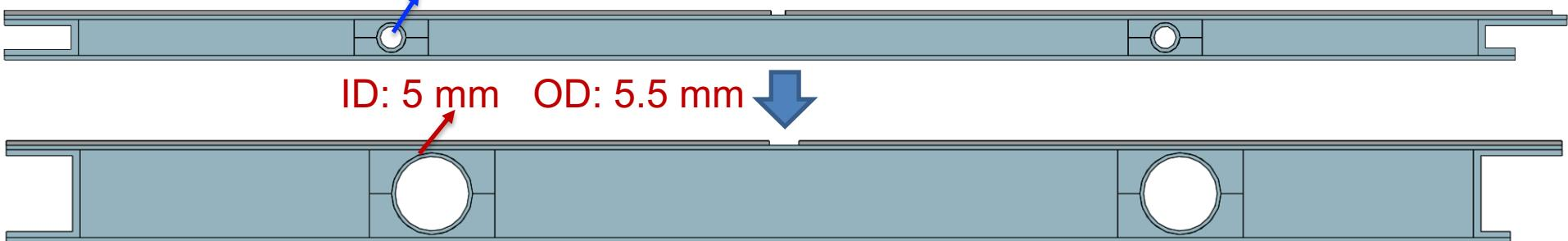
Too small diameter flow cannot meet the cooling requirements, so increase the pipe diameter.
