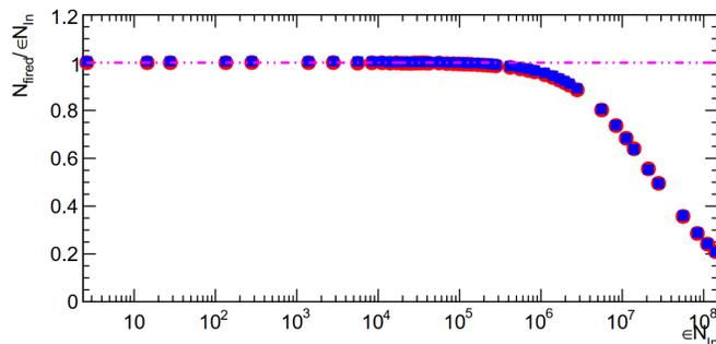
A Monte Carlo model to simulate the SiPM response to BGO(40x40x1cm) scintillation light. The model includes both BGO and SiPM properties.
