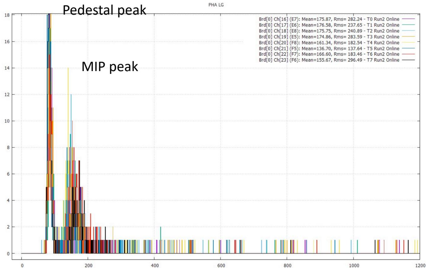
The crystal calorimeter prototype used commercially available ASICs. The S/N ratio is promising and barely noises besides pedestals
