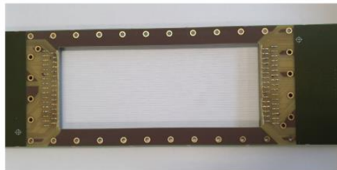
Carbon wire chamber soldered then glued
