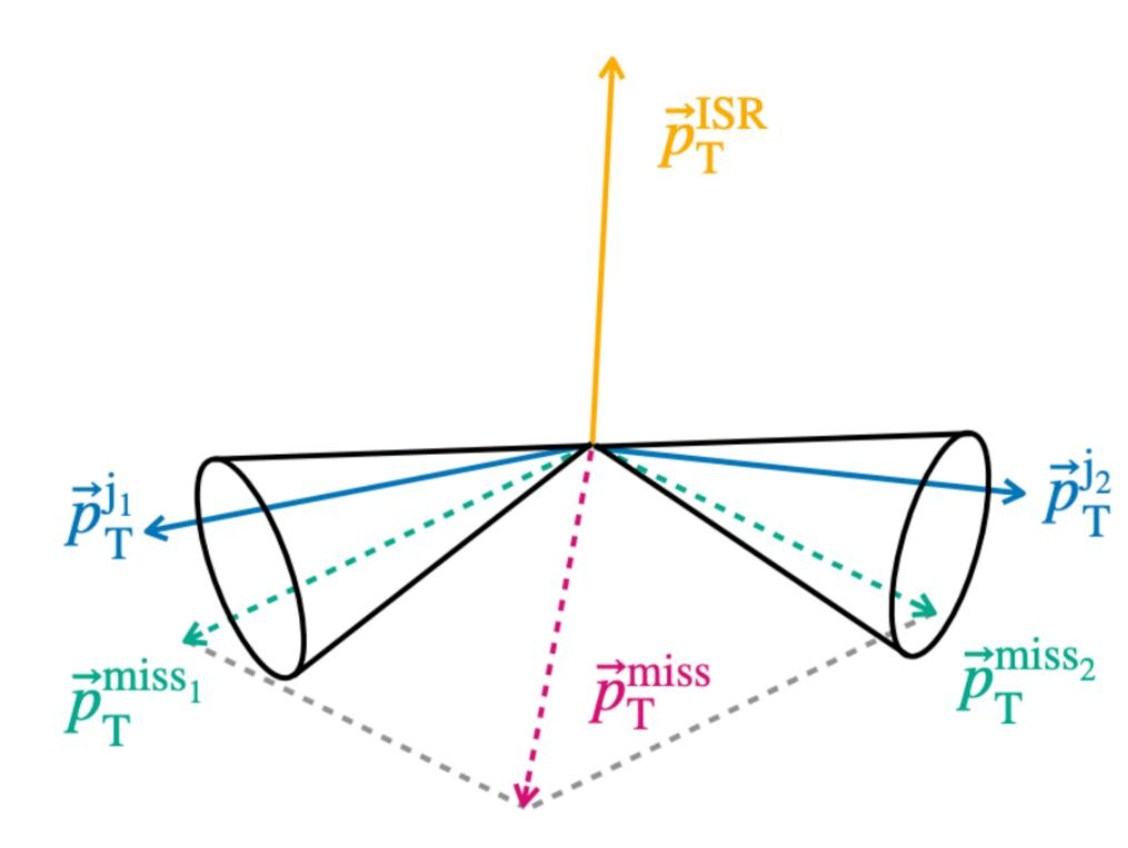
Decomposing the missing energy to the jet axes to approximate the invisible energy
