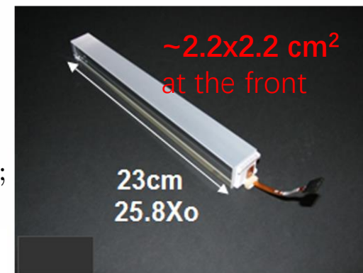
Barrel crystal, tapered 34 types, \sim 2.6 \times 2.6 \text{ cm}^2 at rear
