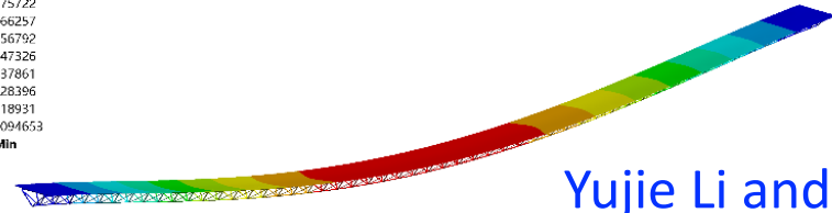
ITKB1 stave deformation
