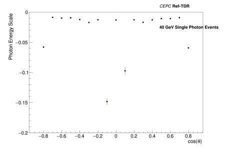
• Cos theta 0.1, 0.8: crack at ecal modules.
