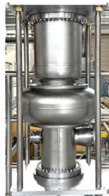
1.3GHz 9-cell, spoke, 166MHz QWR, 500MHz Vertical test reach the state of the art level
